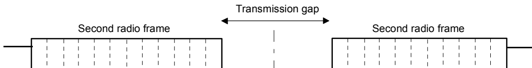
Fig. 24 Envelope of compressed mode signal with double-frame method
